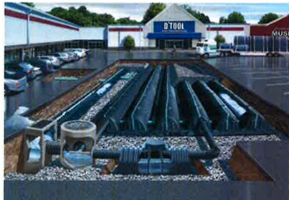
Example of underground storm water system (waterworld.com)
