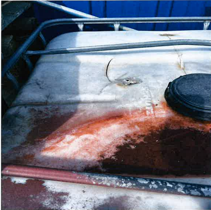
Picture 10: Cracked oil storage container at building J east side.
